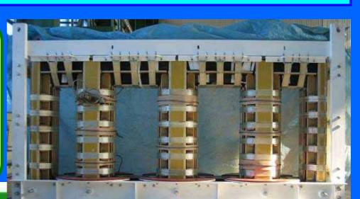
The iron core was made of amorphous alloy.
