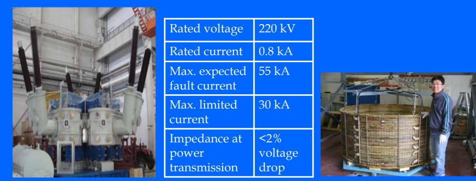
Superconducting coil for FCL
