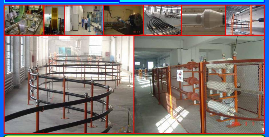
Energized: Dec., 2004 Operation time: more than 7000h.; Critical current of the 75m HTS power: up to 5000A; Joint resistance: as low as  $10^{-7}\Omega$ .
