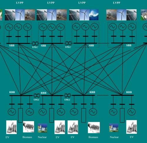
—LVPP: Large Virtual Power Plant —TPEC: Two-way Power Exchange Control —SBB: Super Busbar
